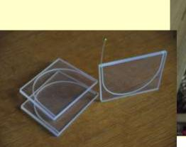
Active elements of the end-cap hadron calorimeter in the CMS experiment
