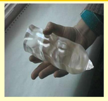
The PWO crystal is a high density, fast and radiation hard scintillation material.
