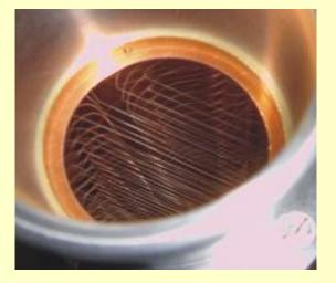
Grid resonator with photonic crystal
